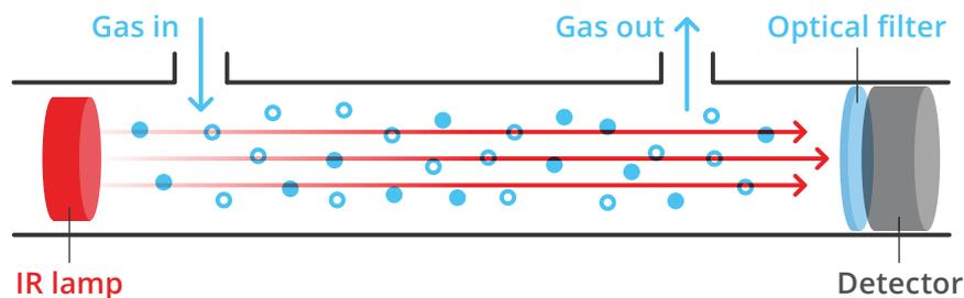
Aranet4 uses the nondispersive infrared (NDIR) sensor to measure the concentration of CO<sub>2</sub>. The CO<sub>2</sub> gas in the chamber absorbs infrared light and this absorption is measured by the sensor. The less light passes through – the higher the CO<sub>2</sub> concentration. The CO<sub>2</sub> gas absorbs only a specific wavelength of the light therefore an optical filter is used.
